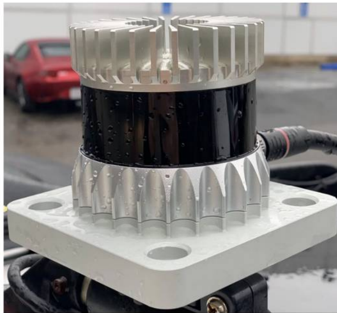
Here's what the lidar sensor looked like at the end of the drive. You can see the water droplets on the sensor window, but they had little to no effect on the sensor data due to the sensor's large aperture.
